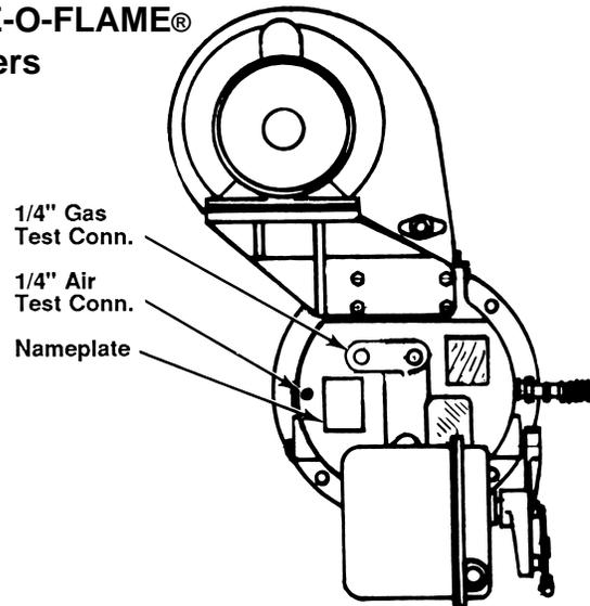
6. **Determine static condition of tube** (draft or suction) and verify differential air pressure at burner backplate air test port. Measure your **air** pressure reading with manometer connected between the burner's **air** pressure test port and atmosphere with the burner at "high fire" position, fuel valves closed, and all air handling systems running.
