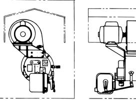
WARNING: Welding of burner flange to a stiffener plate or firing tube may cause warpage of burner flange and require additional seal material to prevent leakage.
