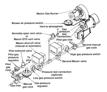
**TUBE-O-FLAME® Burner** provides the air supply (unless it is an LB version, which requires a separate combustion air blower). It also serves as a fuel flow control and fuel/air mixing device.
