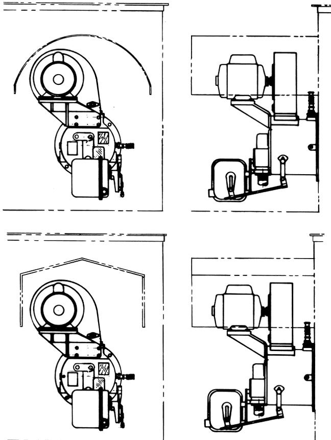
**WARNING:** Welding of burner flange to a stiffener plate or firing tube may cause warpage of burner flange and require additional seal material to prevent leakage.
