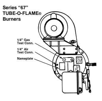
6. **Determine static condition of tube** (draft or suction) and verify differential air pressure at burner backplate air test port.
