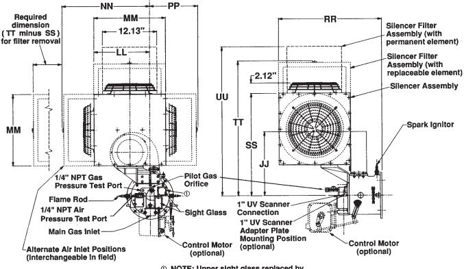
① NOTE: Upper sight glass replaced by UV Scanner Adapter Plate, 1" NPT, if used (optional)
